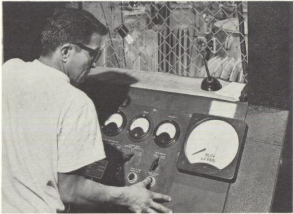
Multi-ampere transformer tester, developed by the company, has saved many man-hours.
