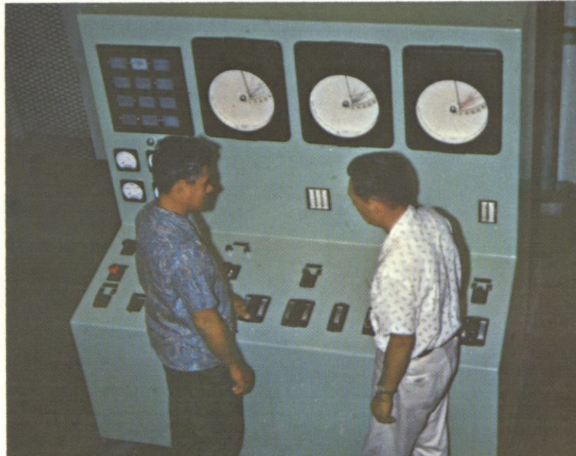
Power plant trainees learn on company-developed "control board" which simulates real conditions.
