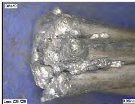
Figure 53: Microscope image of FCA Artifact DB#30, A-Phase dead-end conductor attached to Pole 25 exhibiting melting associated with phase-to-phase fault current
