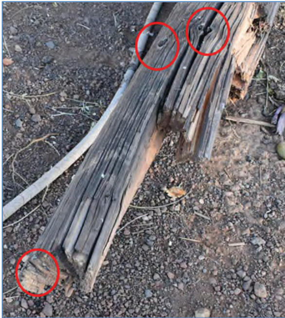
Figure 45: August 13, 2023 field photograph of the bottom Pole 7A fracture surface. For ease of reference, identified knots are indicated by red circles.
